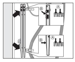
The washing machine must not be moved without the transit bars in place.
